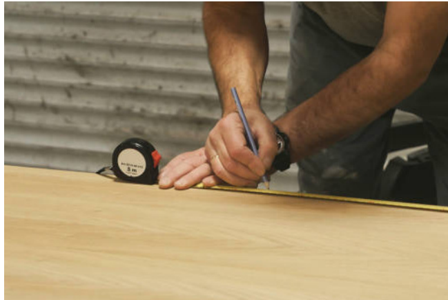
Fig. 1.5.2: marking and measuring boards
