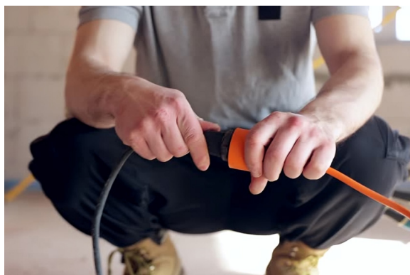
Fig. 3.5.10: Inspect Electrical Cords and Plugs
