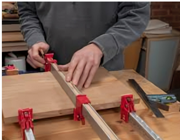
Fig. 3.4.9: Using supports for longer or wide boards
