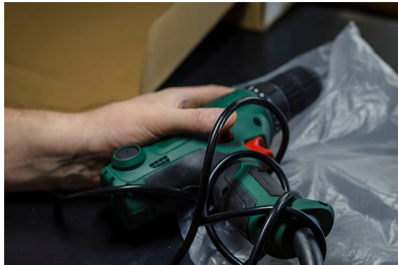
Fig. 3.5.9: Check Power Tools for External Damage
