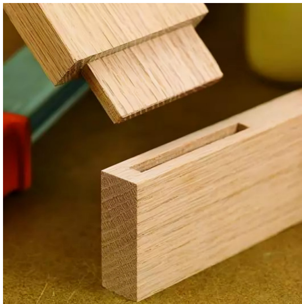
Fig. 6.2.5: Mortise and tenon joint
